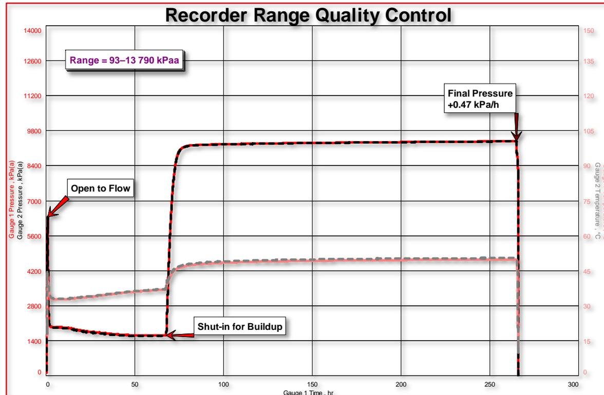
This example is Cartesian plot type #3: scaled relative to the recorder range, 0 – 14 000 kPa in 1400 kPa steps ( $\approx 10\%$ ). 93 kPa is the standardized atmospheric pressure for calculating and reporting in Alberta, Canada.
