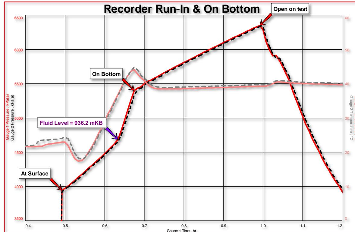
Running speed (m/s) can be estimated by the time difference between surface and on bottom. Interface depths (m) can be estimated, and fluid/gas gradients (kPa/m) can be calculated.
