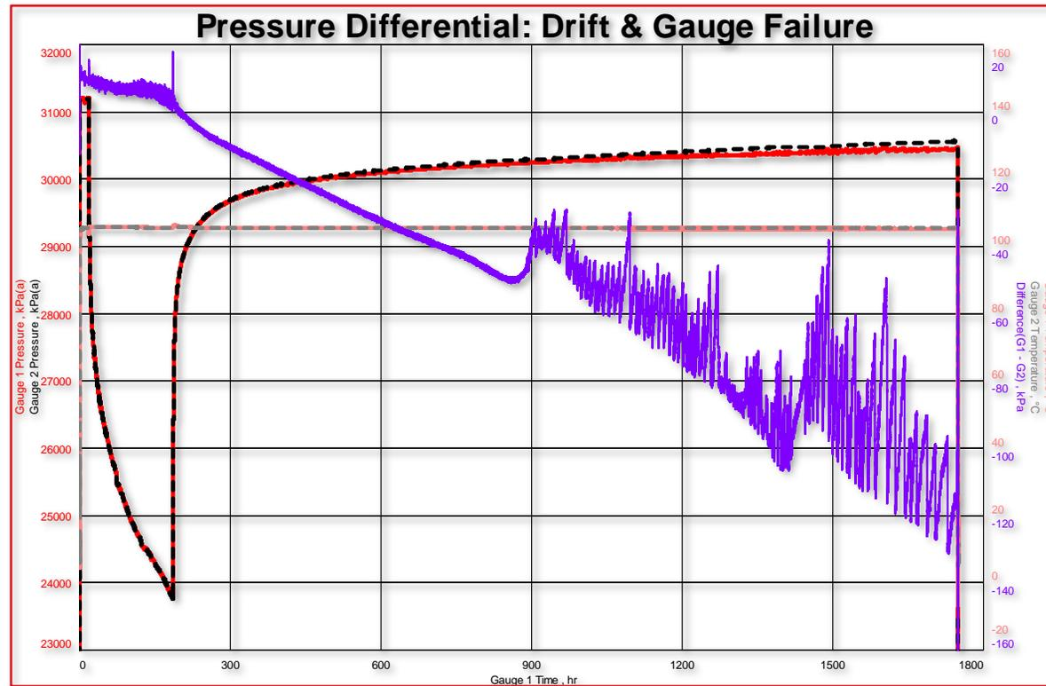
This example is Cartesian plot type #2: relative to test pressures, X lowest measured flowing pressure ( $p_{wf}$ ) to Y highest measured pressure, Y axis = 23,000 – 32,000 kPa.
