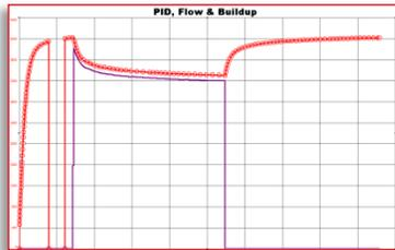
Closed-chamber tests have been utilized for many years as an alternative to drill stem tests. The valve open impulse technique is transferable to several alternative welltest solutions.
