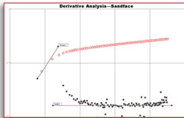
Validity of the technique is demonstrated by two illustrations. This example flow and buildup test was conducted on a 350 m deep low-density sweet gas well with both subsurface and surface electronic pressure recorders installed. The first pressure derivative plot is from the *subsurface data*, the second from the *surface data*. Quantitative analytical results from the two methods ( $kh$ ,  $s'$ ,  $q_s$ ,  $p_R$ ) were virtually identical.
