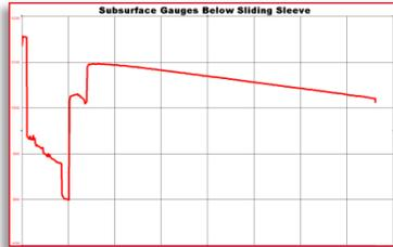
Sometimes using surface pressure data is the only practical testing method available. This example illustrates a test where downhole gauges were set *below an open sliding sleeve* that was *above the perforations*. Valid pressure transient data were totally obliterated by liquid interference. Quiet-side (annulus) surface pressure data may very well have provided valid pressure transient data in this case.
