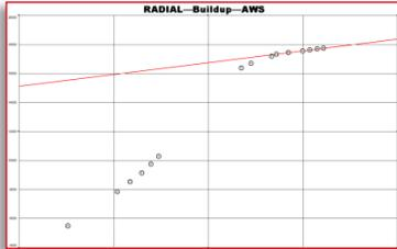
It is common practice in pumping oil wells to use acoustic well sounder (AWS) instruments to obtain reservoir pressure buildup data without pulling rods and pump. With this method each pressure measurement is tied to a liquid level shot, which becomes the primary input signal. Sparse sample rates and noise (due to inaccuracy of the acoustic shot) are inherent problems. Both deficiencies can severely affect pressure derivative analysis techniques.
