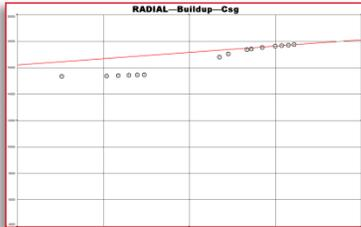
Testing a hypothesis, a number of historical AWS tests were reviewed, evaluating *only* surface casing pressures. Analytically it was presumed that the period of active liquid movement, after shut-in, was a function of wellbore storage (afterflow). The analyzable portion of the buildup was, thus, after liquid movement stabilized, in which case one final static liquid level measurement (AWS shot) should be sufficient.
