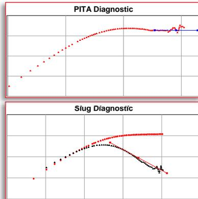
Modern analytical techniques to estimate order-of-magnitude reservoir flow characteristics ( $kh$ ,  $s$ ,  $q$ ,  $p^*$ ) have been programmed into some Welltest software (IHS). Slug, PITA, or Closed Chamber (CC) diagnostics can be performed for build-up, fall-off, or leak-off scenarios. Closed chamber analysis allows for a change in wellbore storage after setting a bridge plug to reduce wellbore volume.
